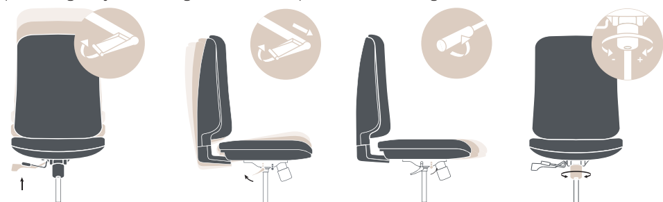
Front right lever adjusts the seat depth
