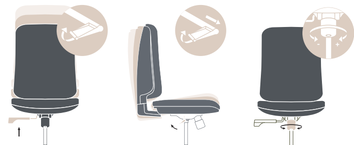
Right lever adjusts the height of the seat
