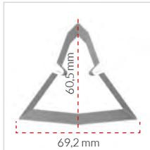
Legs made from 2mm triangle-shaped steel tube, 60.5x69.2mm section.
