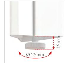
0-15mm adjustable levelling feet made of polyethylene, 25mm diameter.
